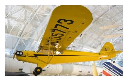
Length: 22'2" Height 6'8" Wingspan: 35'2" Max speed: 85 mph Cruising speed: 75 mph Range: 190 miles
