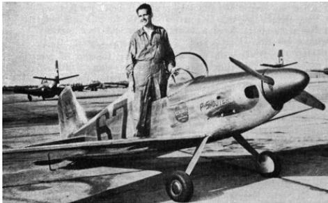
It became known as the Midget Mustang in 1949 after the prototype received a new canopy, wheel pants, and a few other refinements. Designed around the Goodyear Midget Racing specifications it has a wing area of 69 sq. ft. , a racing empty weight close to 550lbs using the 190 cu. in. Continental engine (C-85), and a structure that can take a 6g pull up at 175mph and speeds of up to 260mph.
